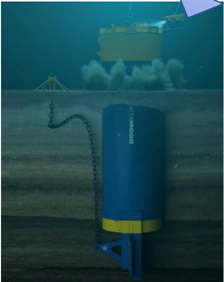
Suction embeded plate anchor (SEPLA) installation process
