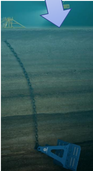
Suction embeded plate anchor (SEPLA) installation process
