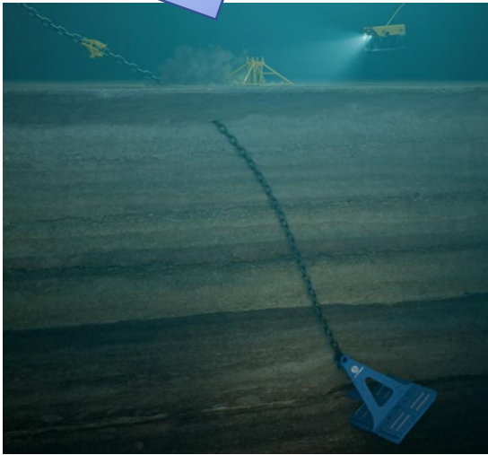
Suction embeded plate anchor (SEPLA) installation process
