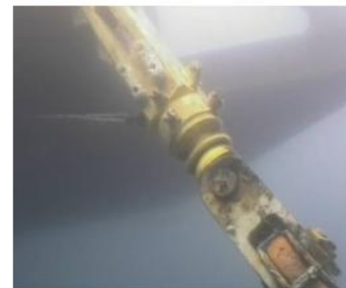
6. Mooring connector automatically locks
