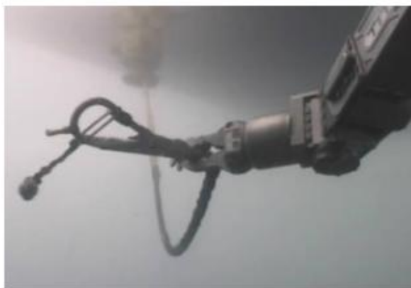
4. Retrieve winch rope with ROV & connect subsea
