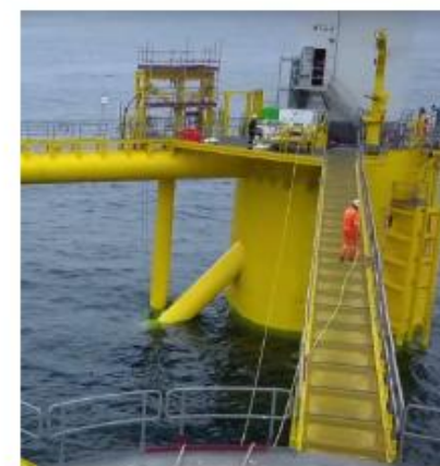
6. Mooring connector automatically locks
