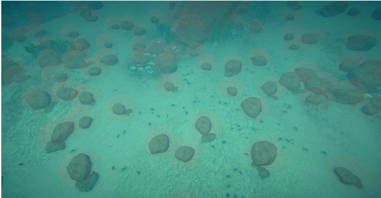
Figure 5 – An object avoidance experiment in OceanViz showing the detailed bottom. Here, crabs roam the sandy habitat but must avoid the rocks. The avoidance buffer is drawn in red for testing purposes.
