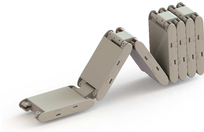
Fig. 3 Modular battery stack concept: Li-ion cells packaging and connectors
