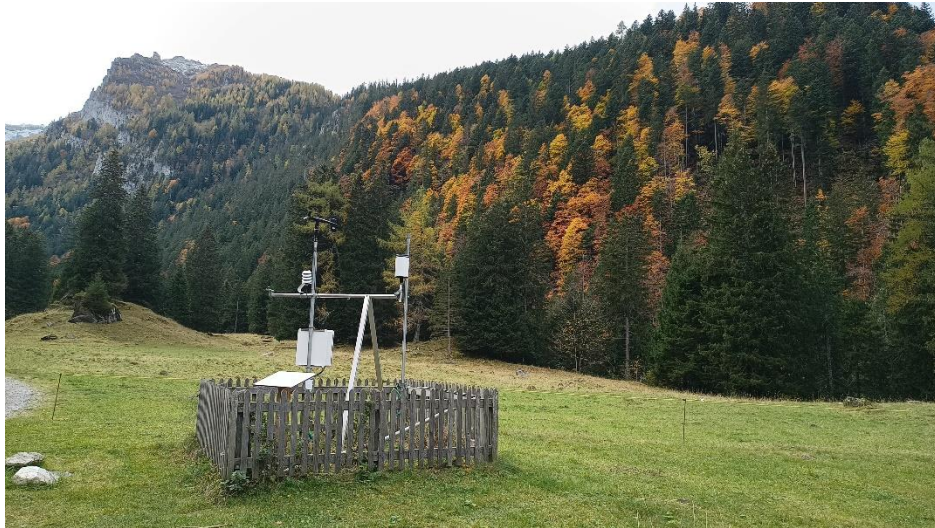
Figure 2. Auberge weather station with additional ultrasonic snow height sensor.
