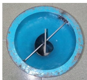
Figure 4. (a) Installation of the swirl generator, (b) Front view of the nozzle with swirl generator
