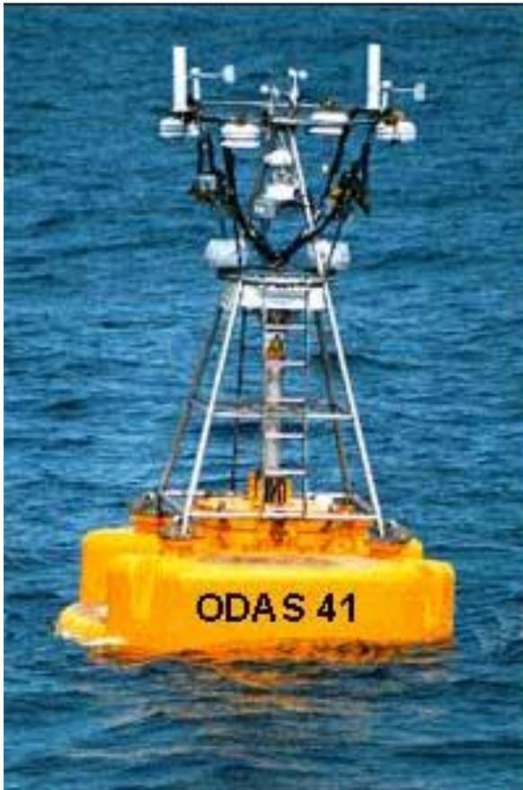
Fig. 3: Met Éireann ODAS buoy, part of the Irish Weather Buoy Network, operating from 2000 to 2011 (Met Éireann, 2016).
