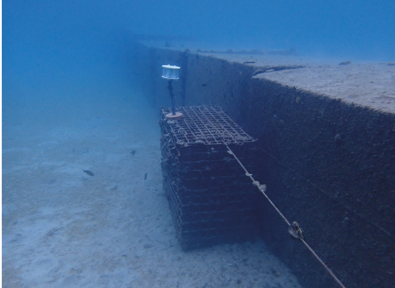
Fig. 8. Sensor installed on top of an oyster cage that is part of the artificial reef experiment "Poseidon's Garden" Fig. 8. Sensor instalado sobre una jaula de ostras que forma parte del experimento de arrecife artificial "Jardín de Poseidón"
