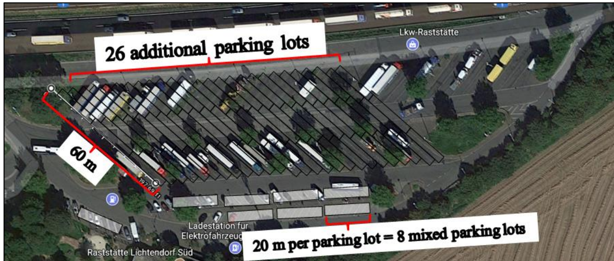
Fig. 4 Example of compact parking and mixed parking analysis (rest area Lichtendorf Süd)
