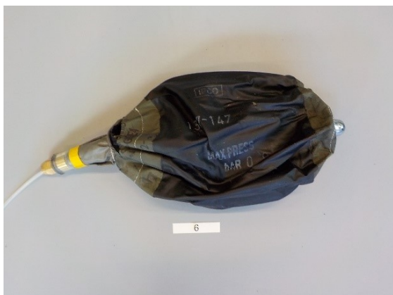
Blaas meting 6; De blaas is gescheurd.
