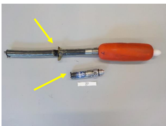
Stopper measurement 26; melt damage at the stopper connection.
