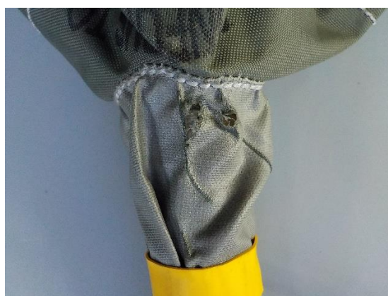
Stopper measurement 11; Fire damage to the stopper or connecting line.
