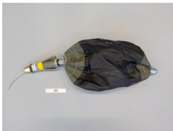
Stopper measurement 65; The stopper is completely ruptured
