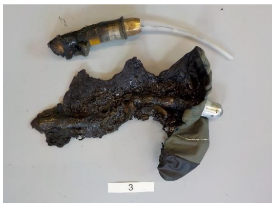
Stopper measurement 3; The stopper is almost completely burned.
