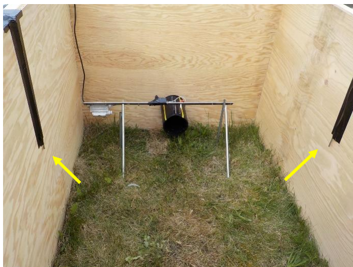
Photo 6 The position of the measuring points for the concentrations in the work pit when extinguishing a natural gas or hydrogen fire
