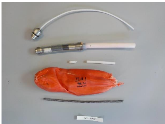
Inner stopper measurement 56; The stopper is ruptured and become detached from the connection.
