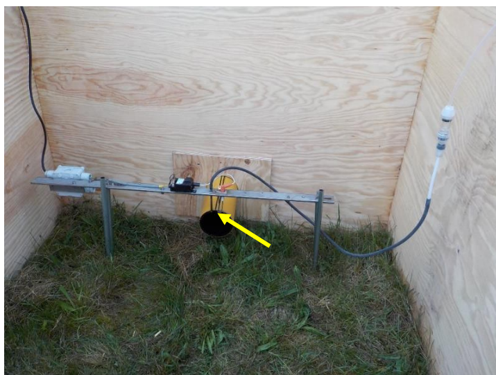
Photo 2 Position of the spark igniter and the measuring point near the outlet opening
