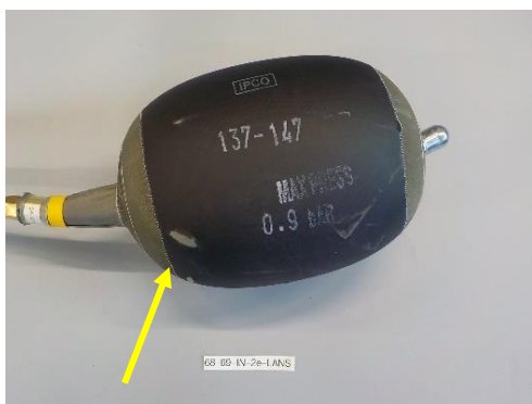
Stopper measurement 69 in inner lance; Cracks in outer layer (at the time of the experiment the stopper was not inflated).
