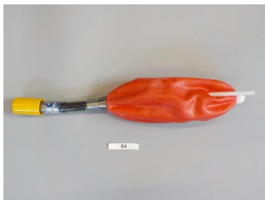
Stopper measurement 64; The filling measuring tube is inserted through the stopper.
