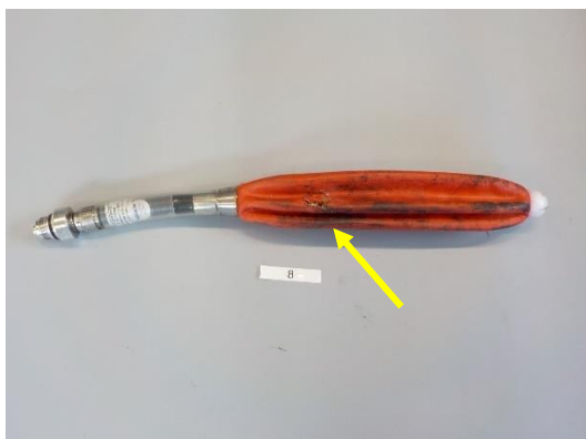
Stopper measurement 8; Burn damage to the stopper and a tear.
