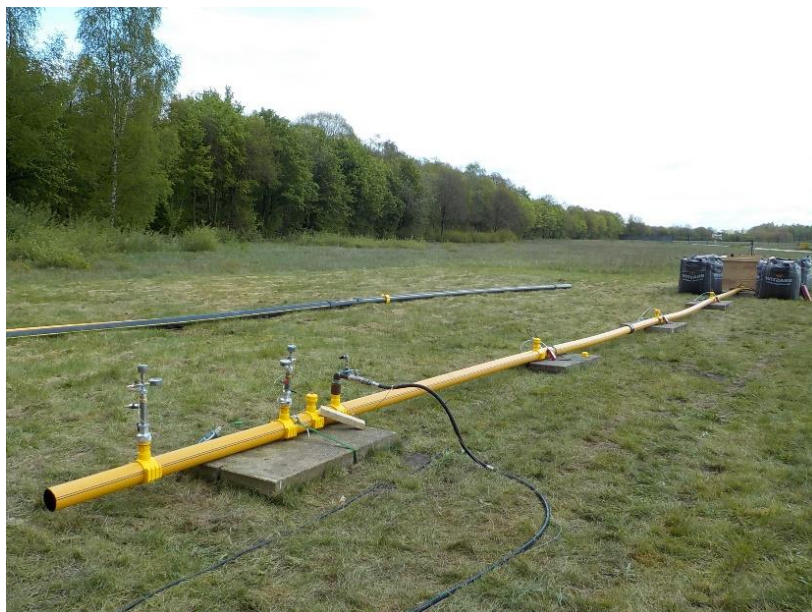
Photo 7 The test setup with the pipe with a diameter of 110 mm containing 2 stoppers.
