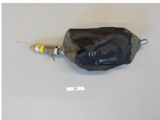
Stopper measurement 35; The stopper is completely ruptured
