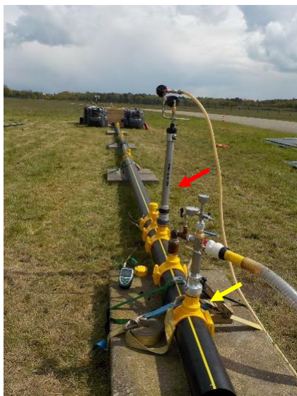
Photo 4 and Photo 5 The measuring setups as used when setting an inflatable gas stopper in the event of a gas fire.
