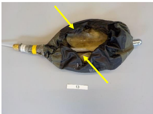
Stopper measurement 13; Completely ruptured stopper due to fire.
