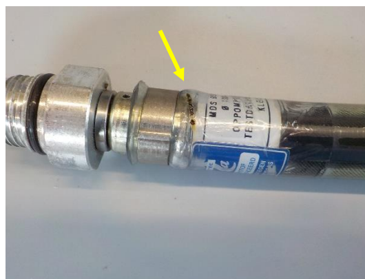
Stopper measurement 9; Melting damage at the stopper connection.
