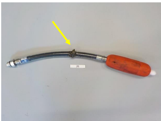
Stopper measurement 26; melt damage at the stopper connection.
