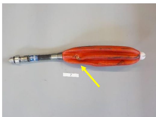
Stopper measurement 7; Burn damage to the stopper and a tear.
