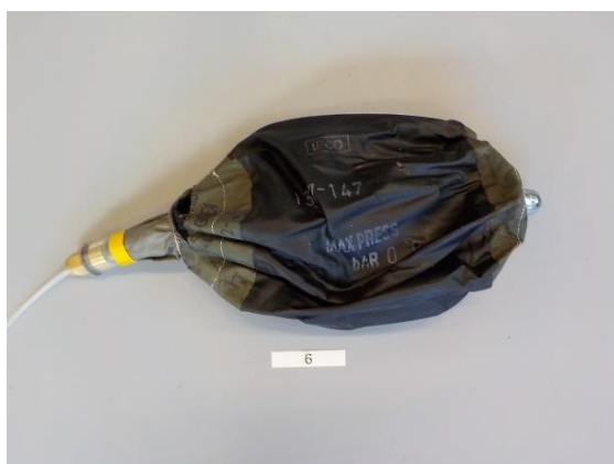
Stopper measurement 6; The stopper is ruptured.
