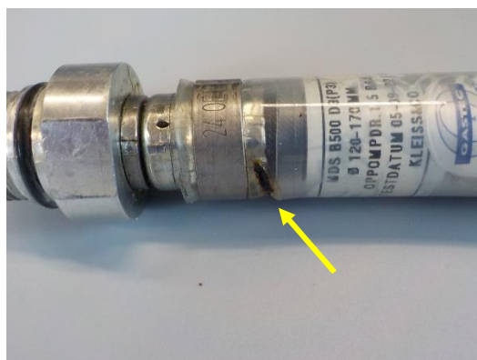
Stopper measurement 8; Melting damage at the stopper connection.
