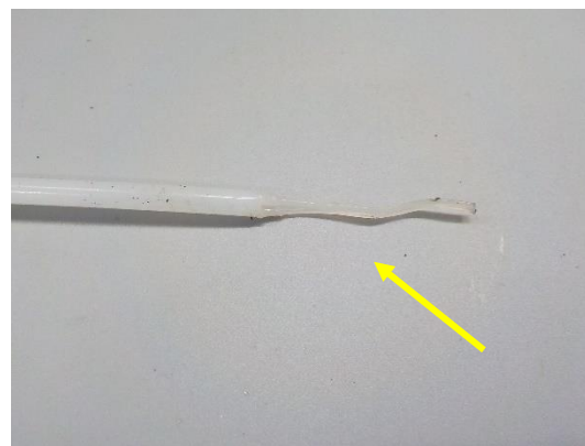
Stopper measurement 28; melt damage - filling tube (internal) melted
