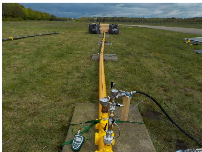
Photo 1 The setup with the pipe with a diameter of 110 mm of 20 meters
