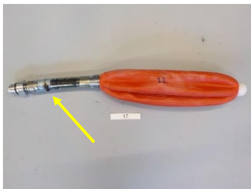
Stopper measurement 17; melt damage at the stopper connection
