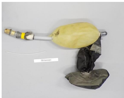
Inner stopper measurement 59; The stopper is completely ruptured (formed as a result of removal from the lance).
