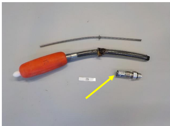
Stopper measurement 29; Melting damage to the stopper connection. This had to be sawn loose to get it out of the lance and pipe.
