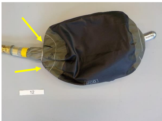
Stopper measurement 12; Fire damage leading to a rupture.
