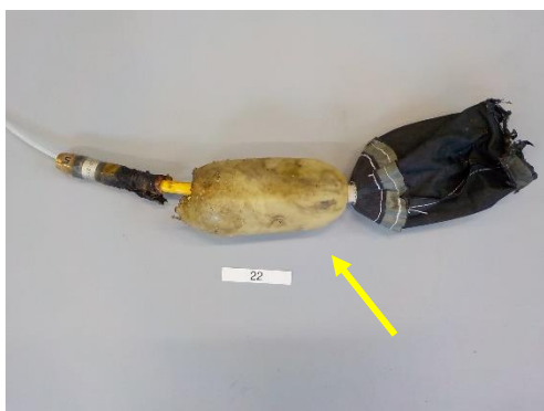
Stopper measurement 22; Completely ruptured stopper due to fire (shaped this way when removed).
