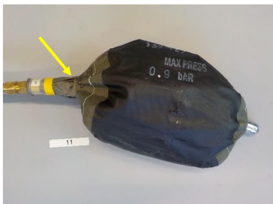
Stopper measurement 11; Fire damage to the stopper or connecting line.
