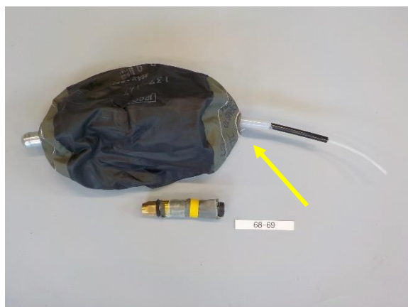
Outer stopper measurement 69; The stopper is completely torn. The connection has become detached from the stopper.
