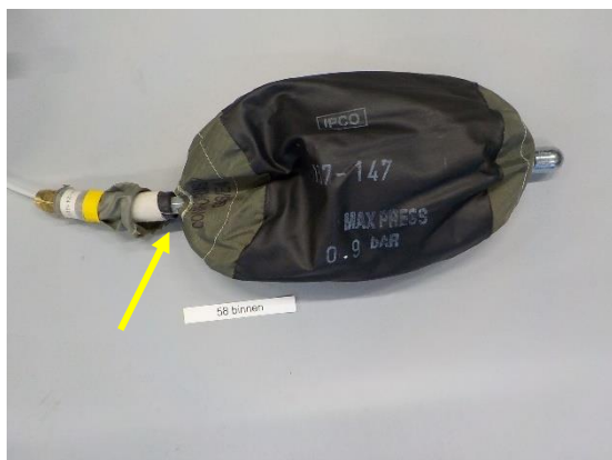
Inner stopper measurement 58; The stopper is completely ruptured.
