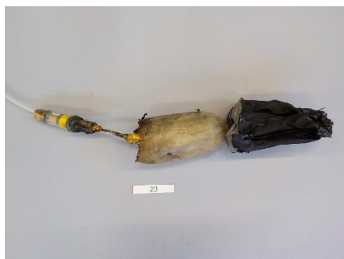
Stopper measurement 23; Completely ruptured stopper due to fire (shaped this way when removed).
