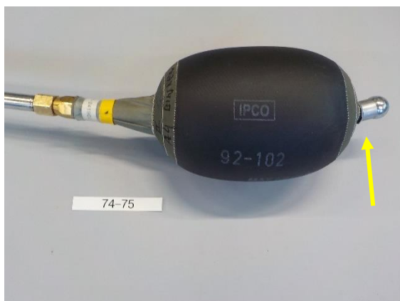
Stopper measurement 70; The stopper is ruptured and become detached from the connection.
