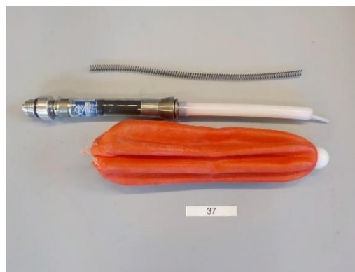
Stopper measurement 37; The stopper is ruptured and become detached from the connection.
