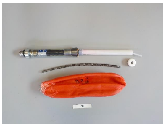
Stopper measurement 70; The stopper is ruptured and become detached from the connection.
