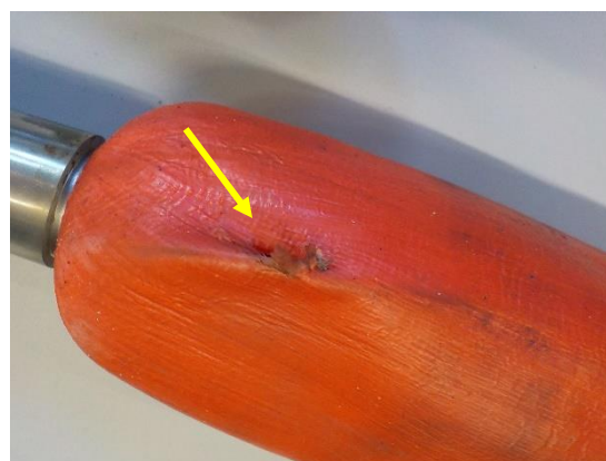
Stopper measurement 27; Burn hole in the stopper.
