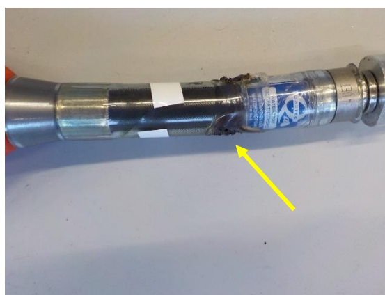
Stopper measurement 14; Melting damage at the stopper connection.
