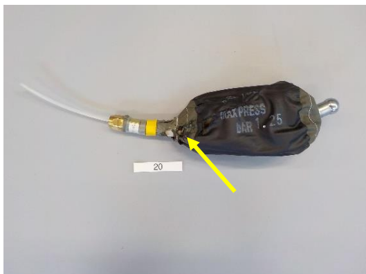
Stopper measurement 20; Burn damage and tear in the stopper.
