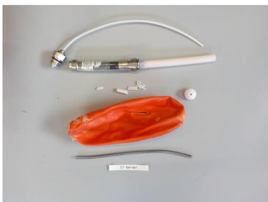
Inner stopper measurement 57; The stopper is torn and detached from the connection. A part of the filling line is broken.
