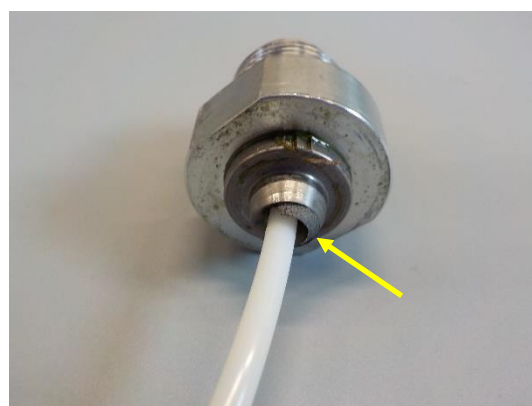
Inner stopper measurement 57; The threaded coupling has broken off the hose.
