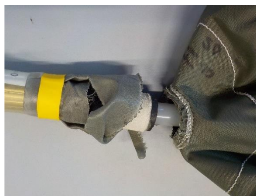
Stopper measurement 35; Detail of the tear.
