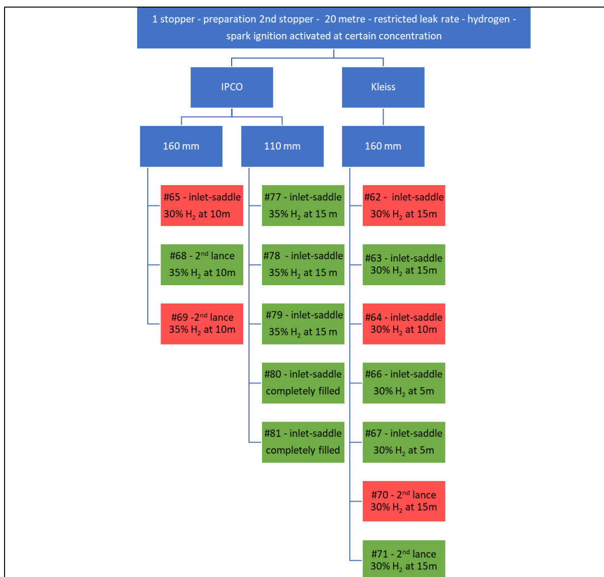
Figure 9 Overview of measurements with preparations for double stoppers in a pipe length of 20 meters
