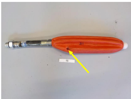
Stopper measurement 16; Burn damage and tear in the stopper.
