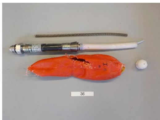
Stopper measurement 36; The stopper is ruptured and become detached from the connection.
