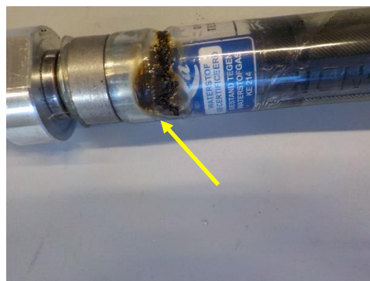
Stopper measurement 16; Melting damage at the stopper connection.
