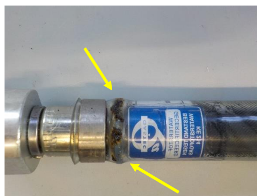
Stopper measurement 7; Melting damage to the stopper connection
