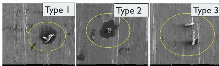
Figure 3. Degradation products forming during the 30-day ageing period and depositing on the surface of the SS316L corrosion coupon
