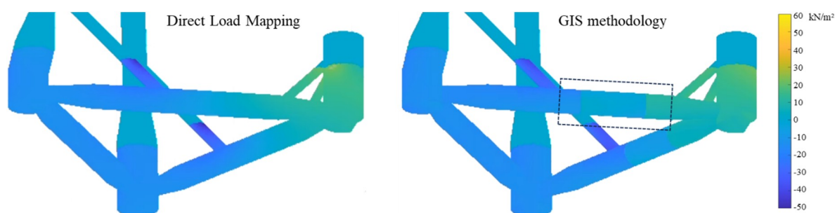
Figure 4. Example comparison of combined wave diffraction, viscous drag and 2 nd -order wave pressures reconstructed by DLM (left) and GIS methodology (right). Only minor discontinuities at the boundaries of the hull segments can be seen in GIS (example marked with rectangle).
