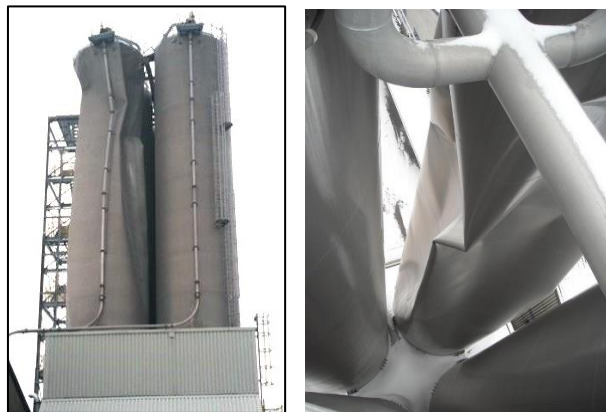
Figure 4. Vacuum damage of a silo during start-up of a closed loop conveying system
