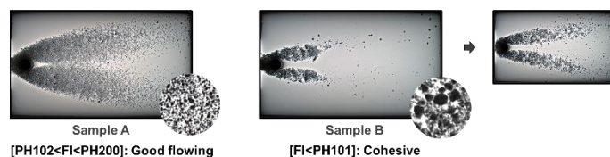
Figure 4. Microdynamic flow patterns. Left: Sample A. Centre: Sample B. Right: Sample B at higher speed. Same magnification for both samples. MCC (PH101, 102 and 200) as flowability reference.
