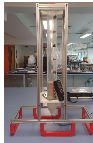
Figure 1. Fluidised bed rig without heating elements
