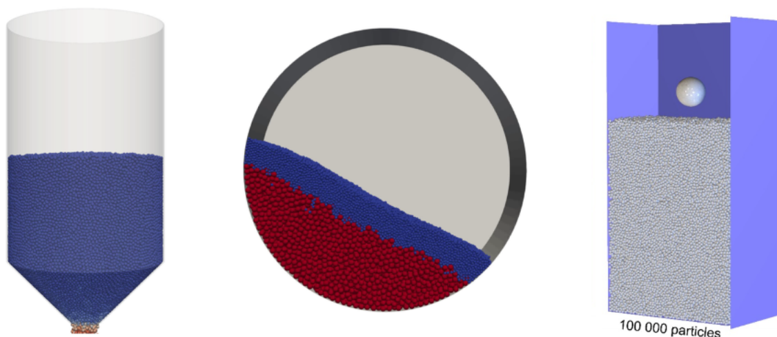
Figure 1: The three common bulk processes, used as benchmarks. Silo emptying (left), drum mixing (centre), and particle impact (right).
