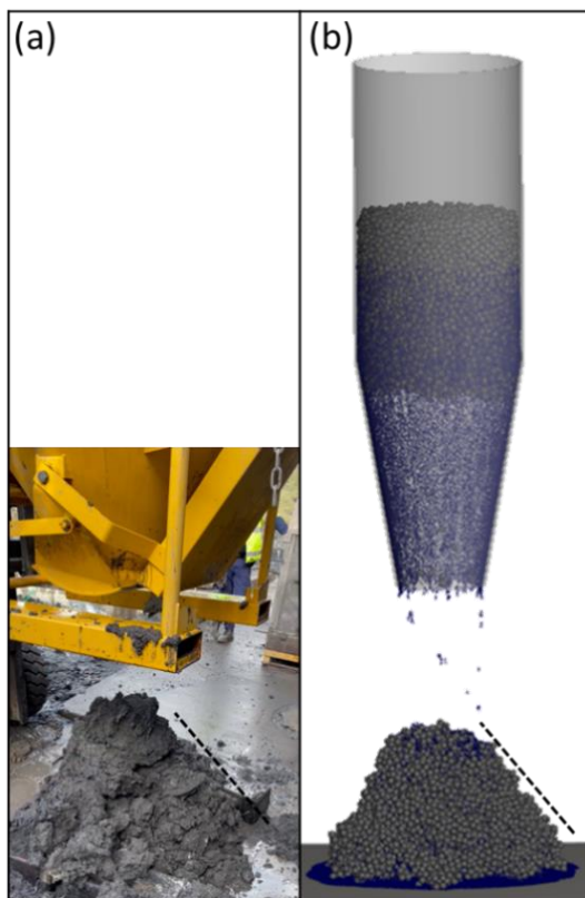
Figure 3: Scaled bin on mine site with a wall angle of 80° and a height of 2.5 m. (a) Experiment, (b) DEM-SPH model.
