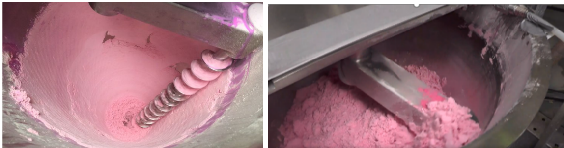
Pictures of the same zeolite under different operating conditions (left) —dominant wall adhesion and (right) —minimal wall adhesion
