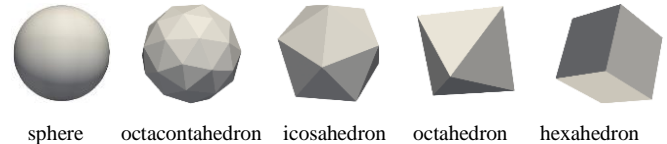
Figure 1. Shapes of particles used for DEM simulations.
