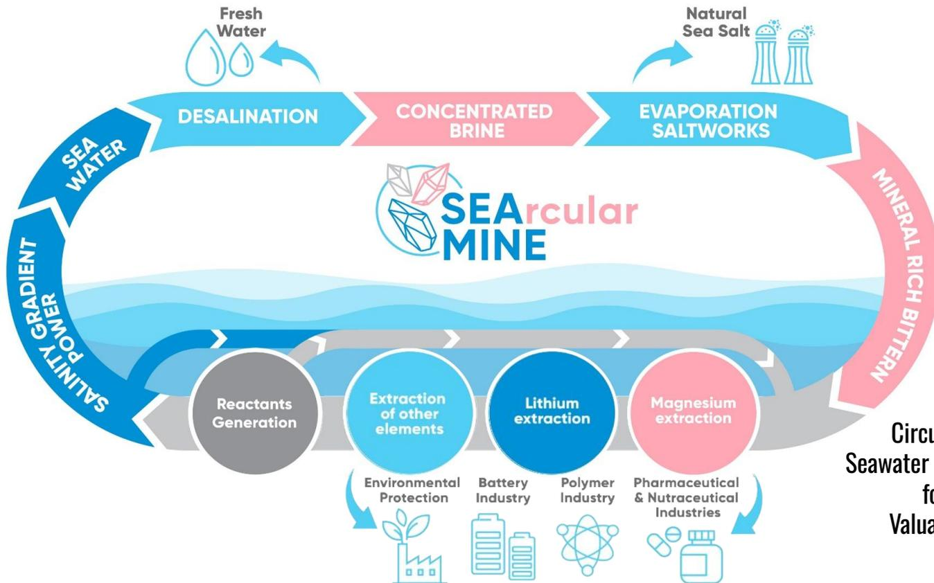
From the original seawater circular mining concept to the integrated pilot plant
