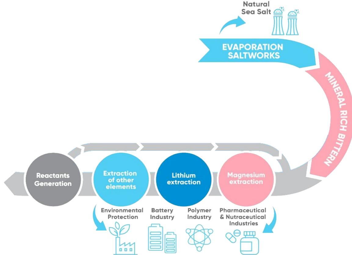
From the original seawater circular mining concept to the integrated pilot plant
