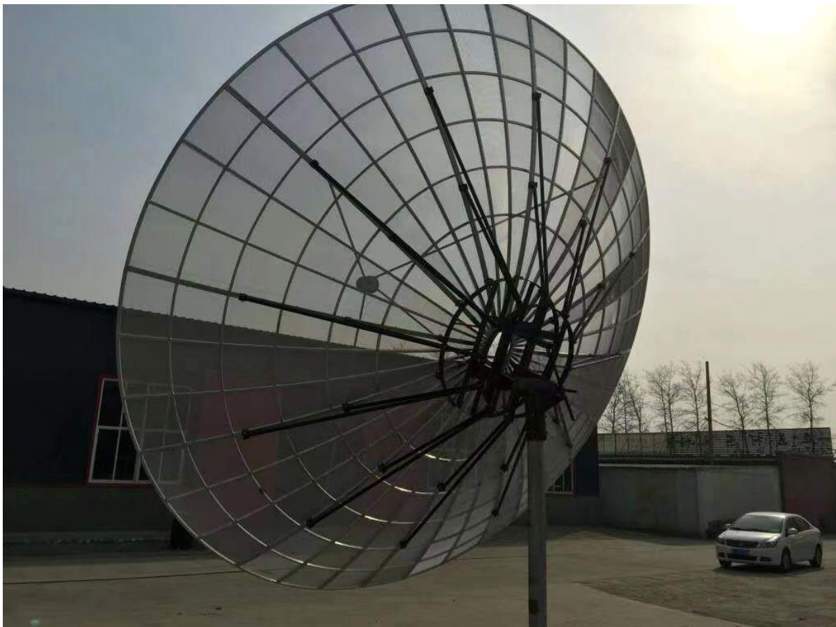
Figure 4-5: Antesky 6m mesh reflector - manual mount.
