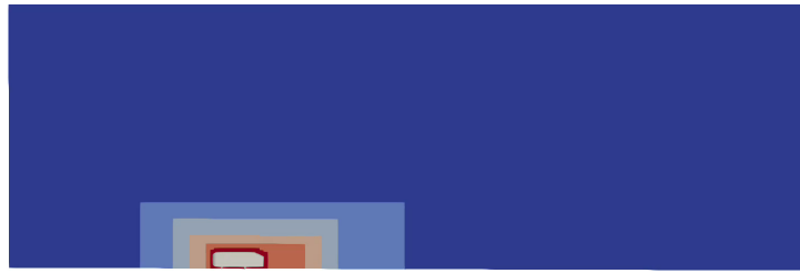
Figure 5: Meshing strategy chosen in the calculation of the flow past the Ahmed Body. Different colours correspond to different levels of refinement. The region coloured in red corresponds to the finest-sampling region, with a lattice spacing \Delta x = 1.3 mm.
