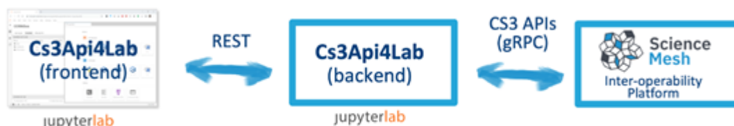
Figure 1. JupyterLab – CS3 API integration back-end component architecture
