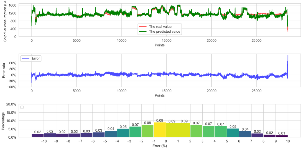
Fig. 20. The error analysis of ship fuel consumption prediction for a whole voyage 1 (In the upper figure, the red line represents the real values of ship fuel consumption, while the green line represents the predicted results. In the middle figure, the blue line represents the error rate in the time domain. The bottom figure presents the prediction error distributions.)
