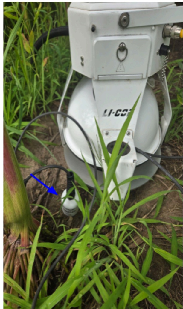
Figure 7: The soil sensor probe (blue arrow).
