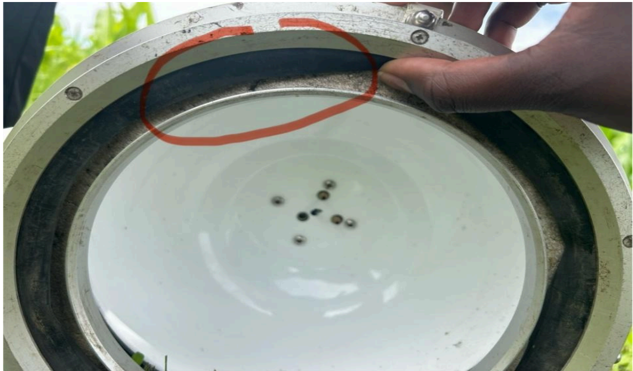
Figure 8: The collar alignment slot and surrounding rubber gasket.
