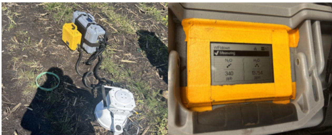
Figure 1 (left) :Analyzer and chamber setup. Figure 2 (right): Analyzer screen
