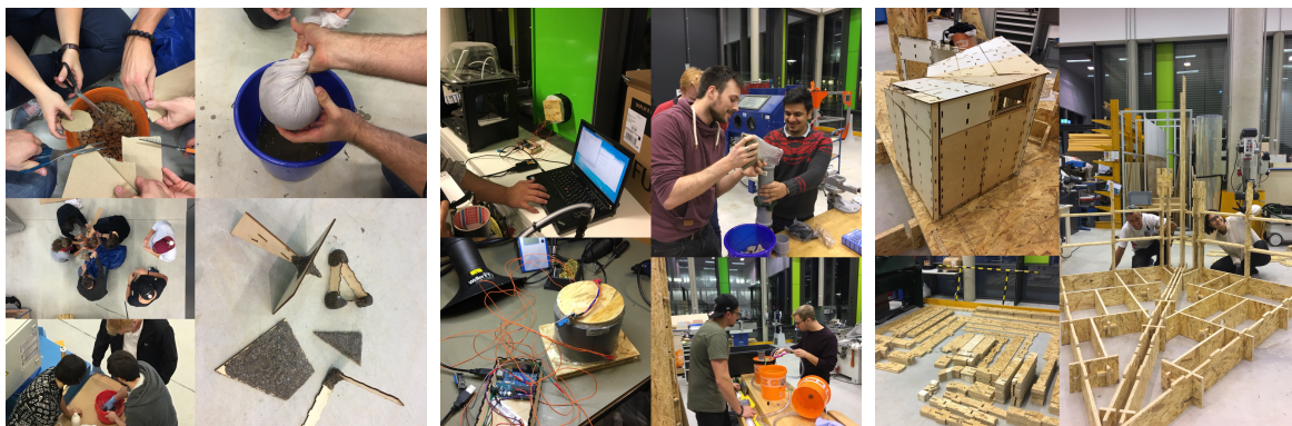
Figure 2: Experimenting with paper clay (left); Setting up the water filtration system, and setting up the bio-gas reactor (middle); Model and assembly of the first life-size prototype (right).
