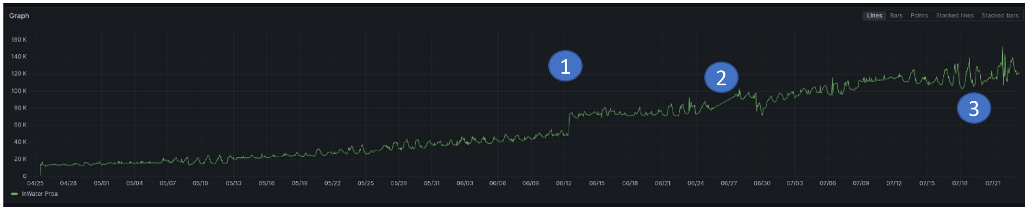
Figure 33. Increase of the weight of mussel rope during. Three events detected by Load cells.
