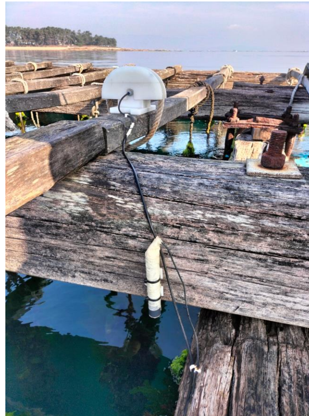
Figure 25. Device for in situ weight control of mussel rope.
