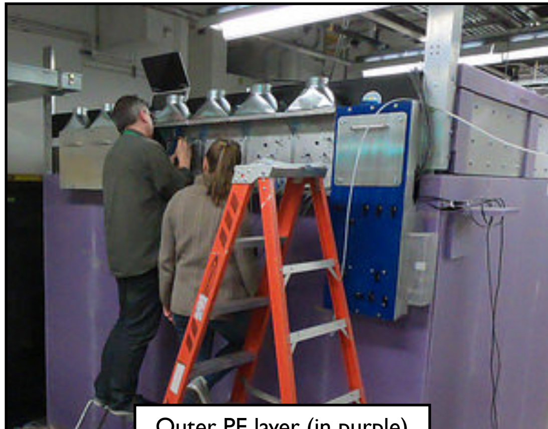
Borated PE shielding under target
