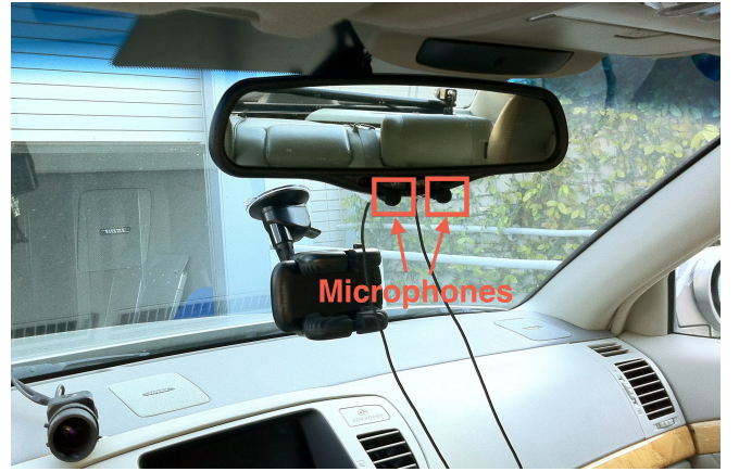
Fig. 3. Microphone setup for data acquisition in LISA-Q. Two microphones are positioned 4 cm apart under the rear-view mirror.
