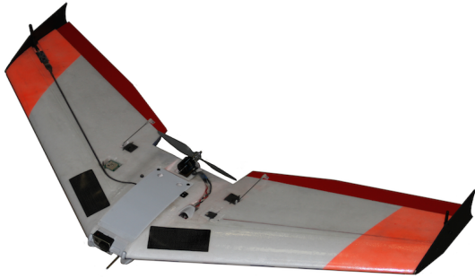
Fig. 1. Picture of NPS Zephyr II UAV, a low-cost yet capable system leveraging open-source and commercially available components [11].
