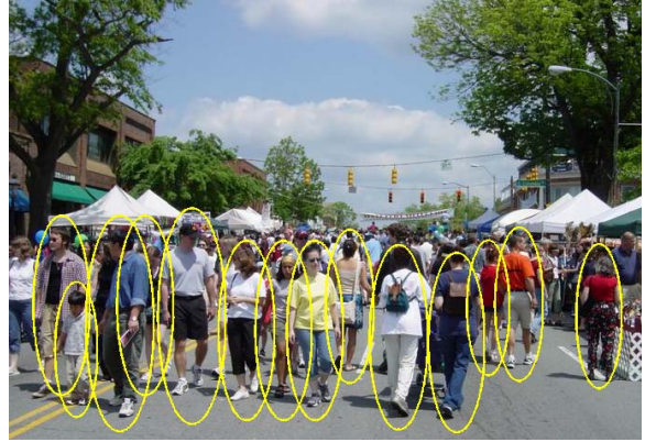
Figure 1. Image demonstrating the performance of our system in a complex scene. The image ( 689 \times 480 pixels) is scanned at 10 scales to search for humans of multiple sizes. We achieve minimal false alarms even though the number of detection windows is 44,996 (best visualized in color).
