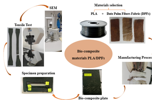
Fig. 3. Manufacturing and testing process.
