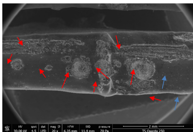
Fig. 8. Adhesion of PLA/DPF-10 interface.
