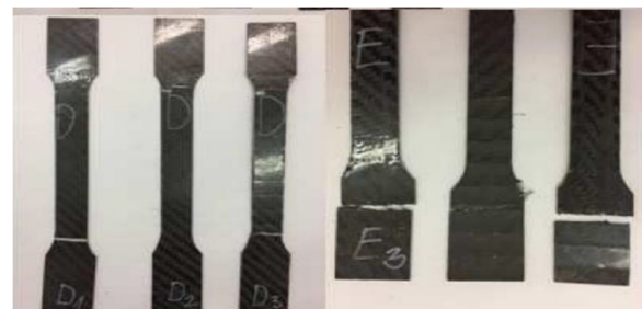
Fig. 7. Broken samples after the tensile test.
