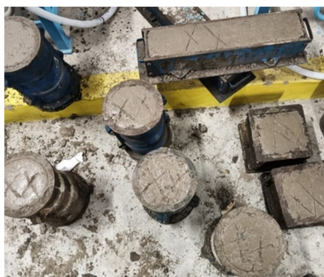
Fig. 5. Temperature curing of GPC specimens.
