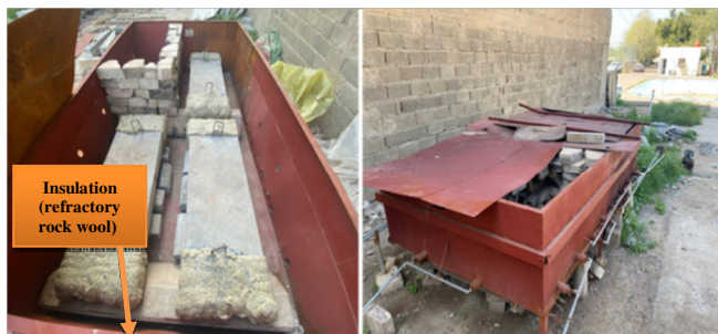
Fig. 5. Setup of the furnace and specimens.
