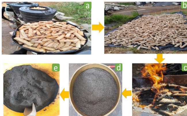
Fig. 2. Treatment and preparation of CCA: (a) Soaking of cobs, (b) drying of cobs, (c) incineration, (d) sieving, (e) ash.
