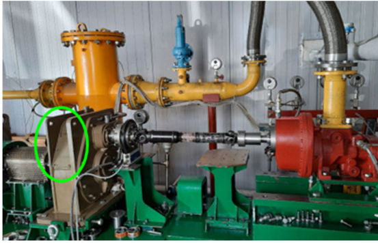
Fig. 3. Optimal screw mounting spot for the TEGs.
