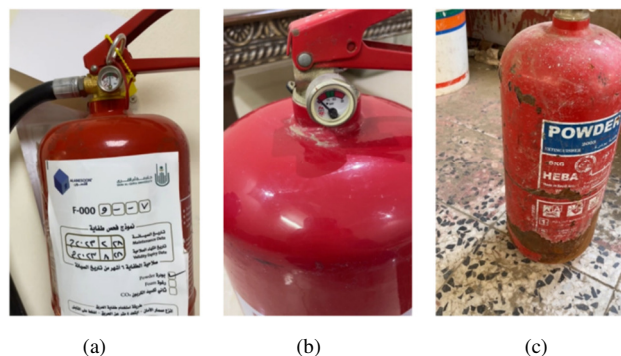
Fig. 2. Dataset examples of defective and non-defective fire extinguishers: (a) Non-defective extinguisher meeting all conditions; (b) Defective extinguisher lacking both safety pin and hose, and the gauge indicator being in the red area; (c) Defective extinguisher showing rust and absence of the hose.
