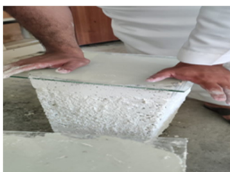
Fig. 4. Pushing gypsum with a flat glass square.
