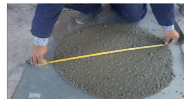
Fig. 3. Slump flow test.
