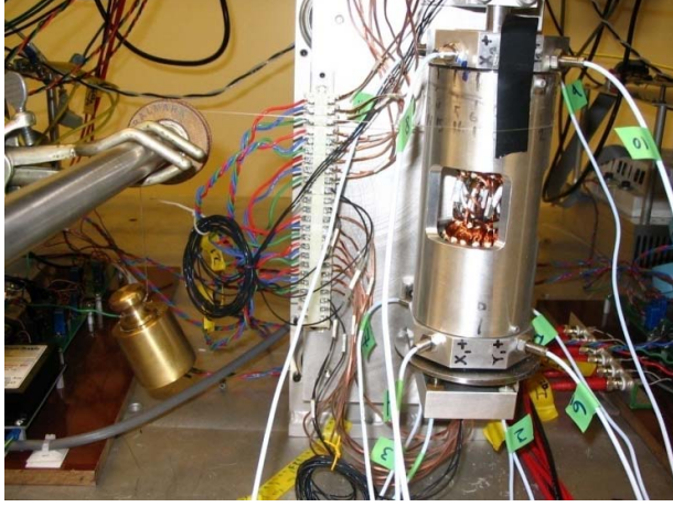
Figure 16: Force Applied to Bearingless Machine
