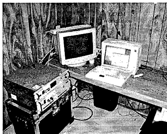
Figure 9. CPDLC Ground Station Equipment
