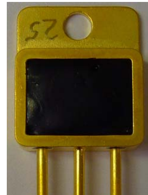
Figure 1. 1200V SiC MOSFET sample from Cree.
