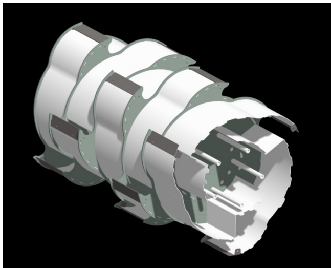
Figure 1 - Bucket drum without end cap to show baffles.
