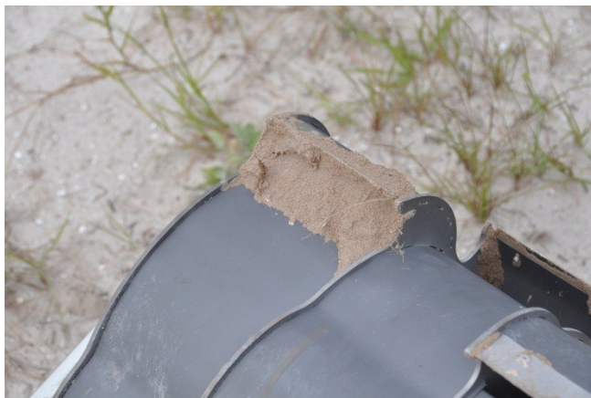
Figure 11 – Scoop clogged with damp sand.
