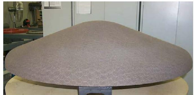
Figure 2. One meter ablative aeroshell with ARA's PhenCarb 20 TPS material.
