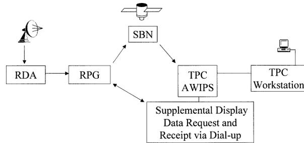
FIG. 1. The flow of WSR-88D display data to TPC. The display data are generated from the base data at the RPG, which are in turn derived from the raw analog data gathered at the Radar Data Acquisition (RDA) site. Display data files are transferred automatically from the RPG to AWIPS via SBN. An AWIPS user may also request supplemental display data from a specific radar site via dial-up to its RPG. The display data are sent from AWIPS to a TPC workstation where the various algorithms are located.
