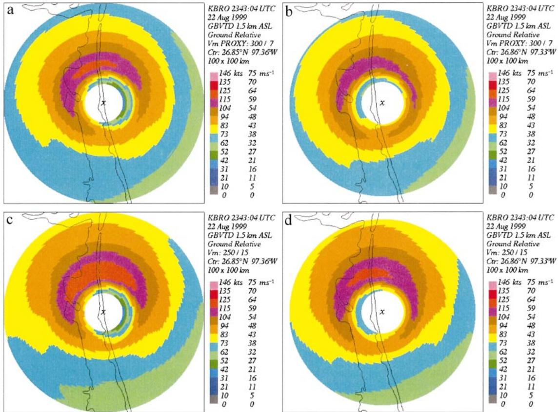
FIG. 9. Same as Fig. 8, except the GBVTD ground-relative wind speed for Hurricane Bret calculated from the KBRO CAPPI map and resolved with respect to the (left) SIMPLEX\_KBRO and (right) PCA\_KBRO circulation centers.
