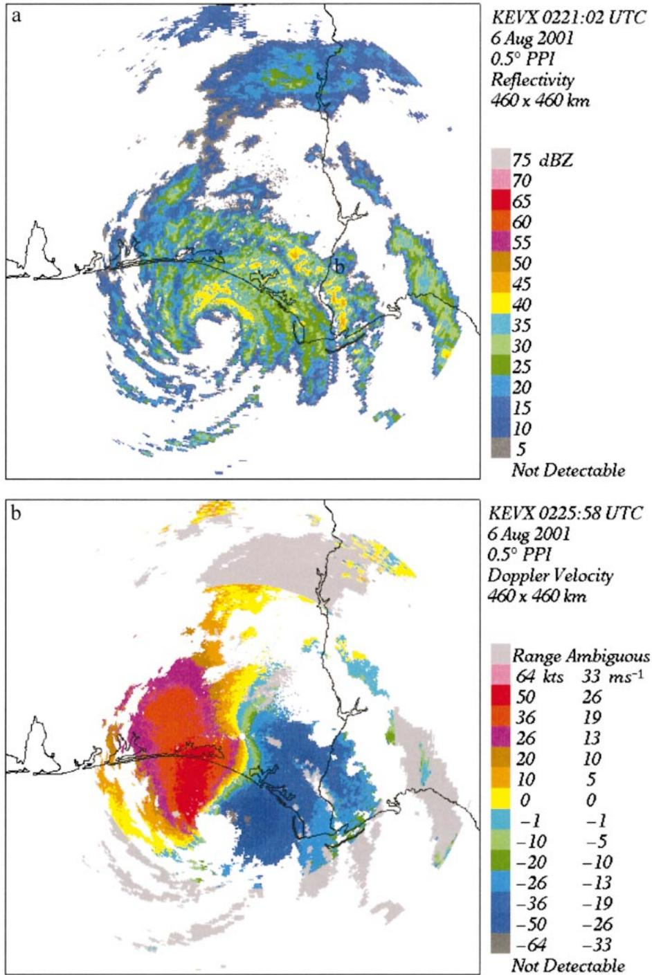
FIG. 12. The 16-contour-level PPI maps at 0.5° elevation showing Tropical Storm Barry as it made landfall along the Florida panhandle near the KEVX radar on 6 Aug 2001. The maps show a 460 km × 460 km area centered on KEVX: (a) reflectivity at 0221:02 UTC and (b) Doppler velocity at 0225:58 UTC.
