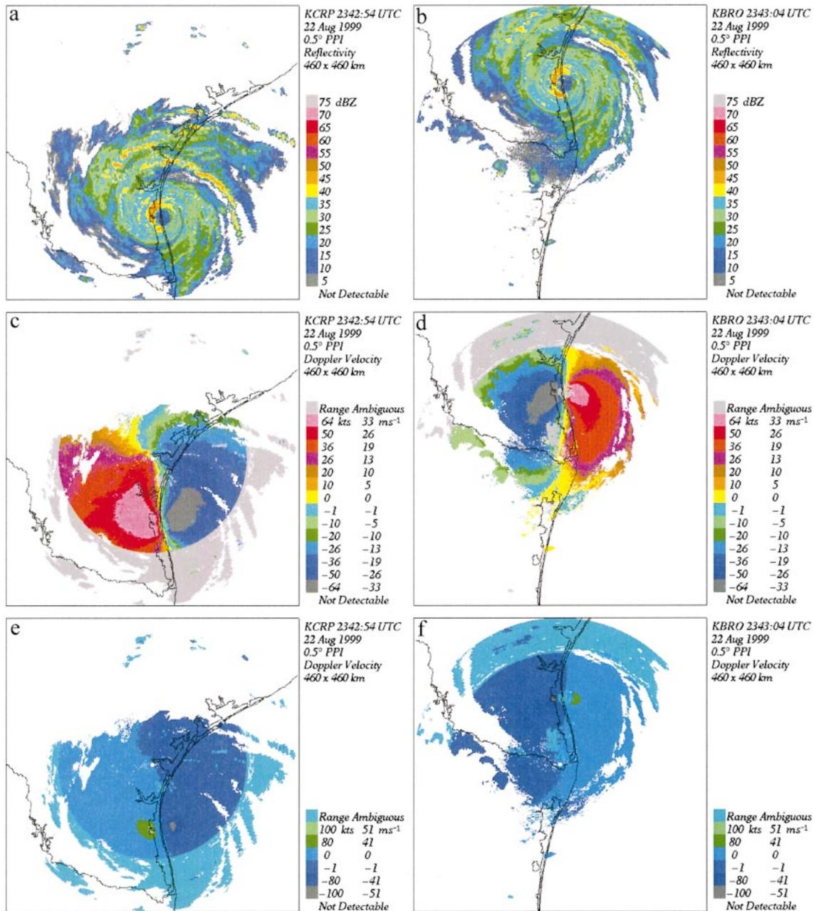
FIG. 4. PPI display data at  $0.5^\circ$  elevation showing Hurricane Bret as observed by (left) KCRP at 2342:54 UTC and (right) KBRO at 2343:04 UTC. (a), (b) The 16-contour-level reflectivity; (c), (d) the 16-contour-level Doppler velocity; and (e), (f) the 8-contour-level Doppler velocity. The particular radar is located at the center of each  $460 \text{ km} \times 460 \text{ km}$  domain.
