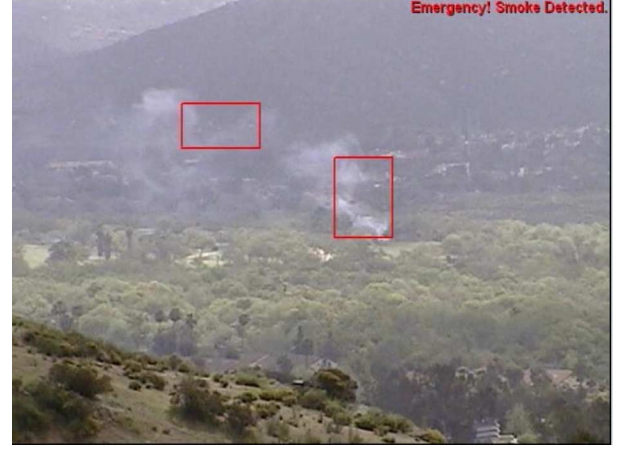
Fig. 5. Photograph from an independent test of the system by the Regional Technology Clearing House of San Diego State University in California in April 2009. The system successfully detected the test fire and did not produce any false alarms. The detected smoke regions are marked with rectangles.
