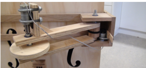
Fig. 2. First bowing mechanism and instrument design
