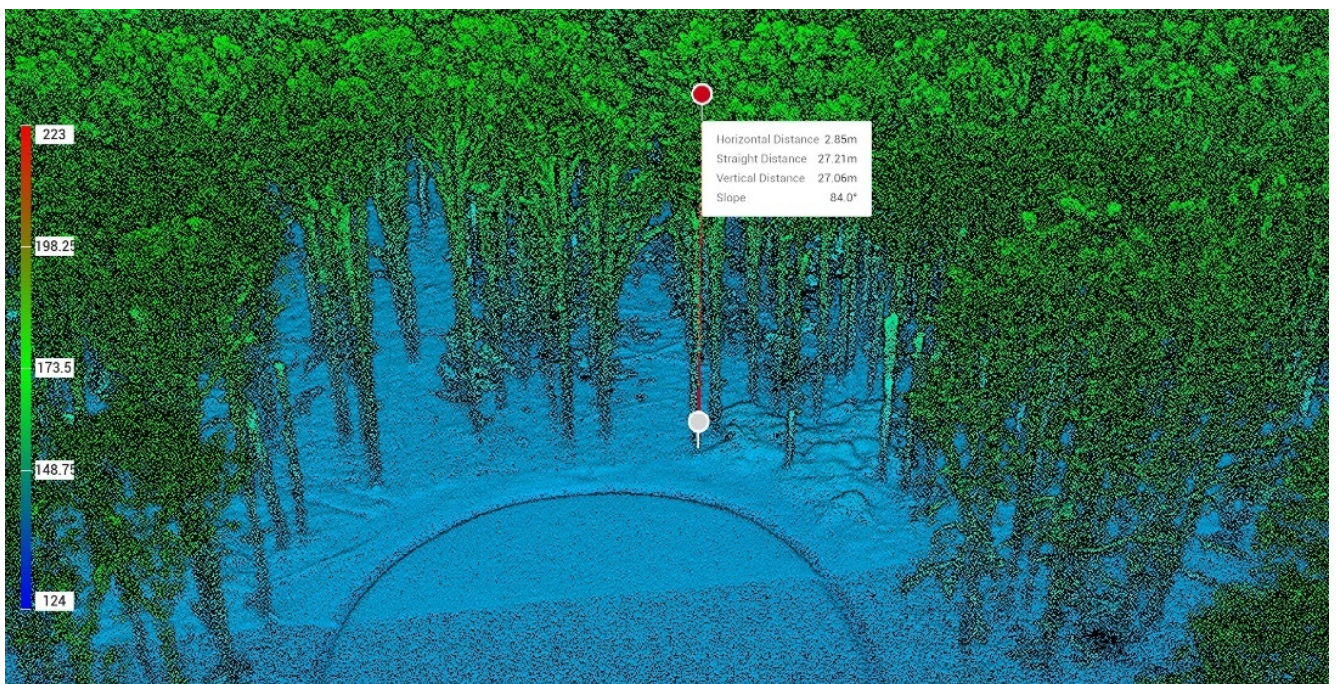
Figure 4. 3D model of an old oak stand taken by a DJI R300 drone equipped with an airborne LiDAR head, generated from a point cloud with a graduated symbology of the height above sea level (courtesy of "Croatian Forests" Ltd.).
