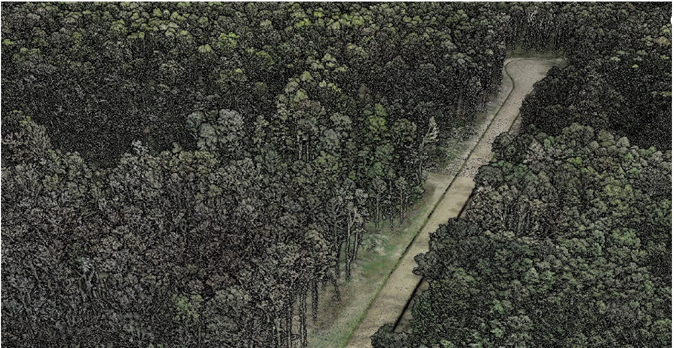
Figure 3. 3D model of an old oak stand taken by a DJI R300 drone equipped with an airborne LiDAR head, generated from point cloud (courtesy of "Croatian Forests" Ltd.).
