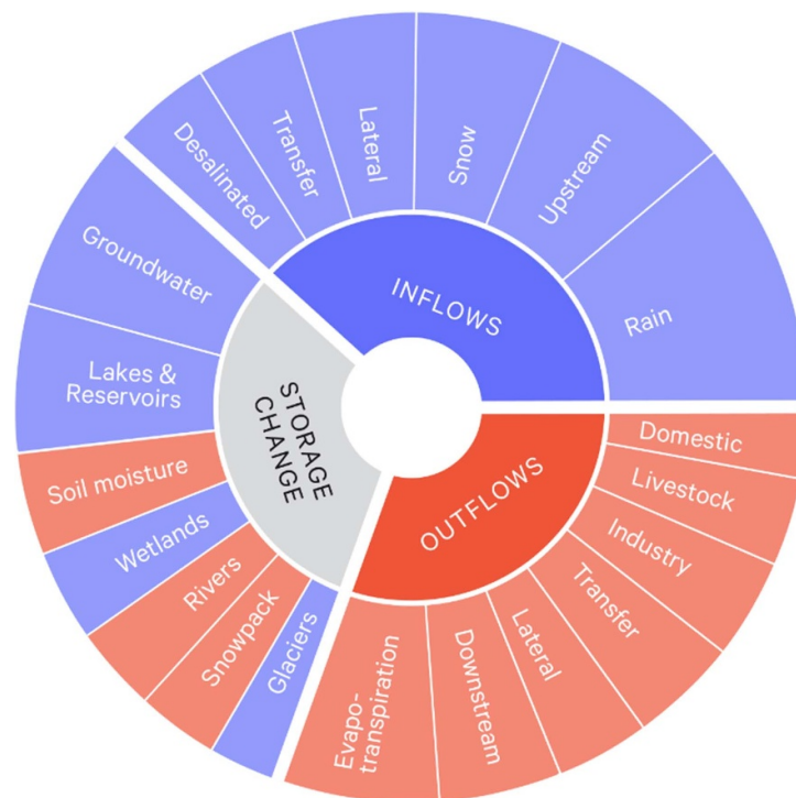
Figure 1. General water circle example. Inflows include the water that entered a specific region/component over a specified period. Storage changes highlight how the different storage components increased (blue) or decreased (red) over the period. Outflows include water that leaves the region/component over the period.
