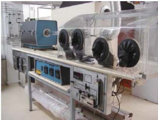
Diffusion furnace (GaSb cell fabrication)
