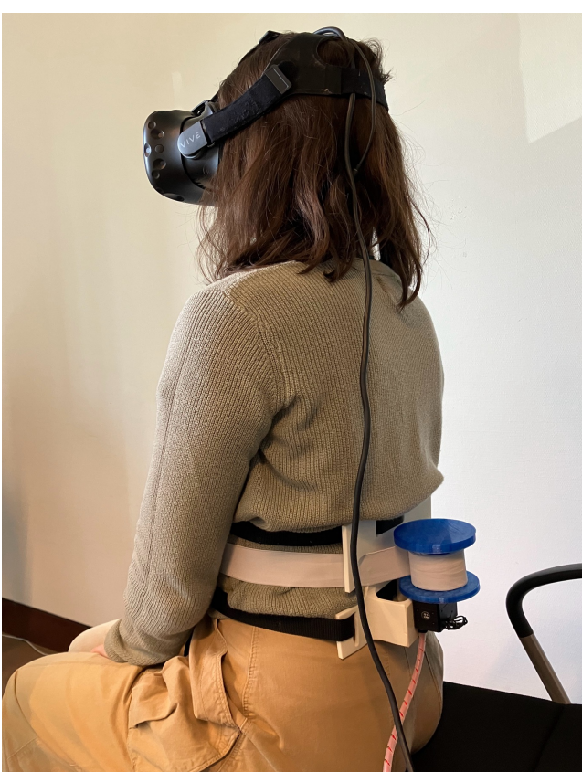
Figure 2. Haptic stimulation belt
