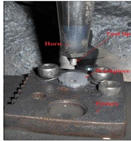
Fig. 1 Machining zone
