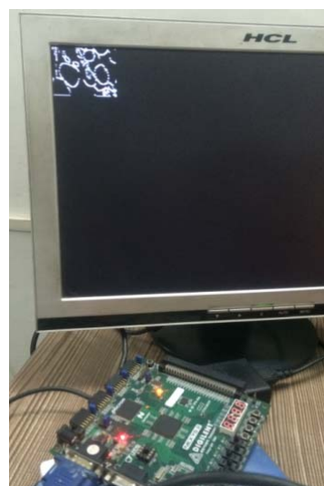
Fig. 9 VGA screen with Xilinx Vertex 4 development board
