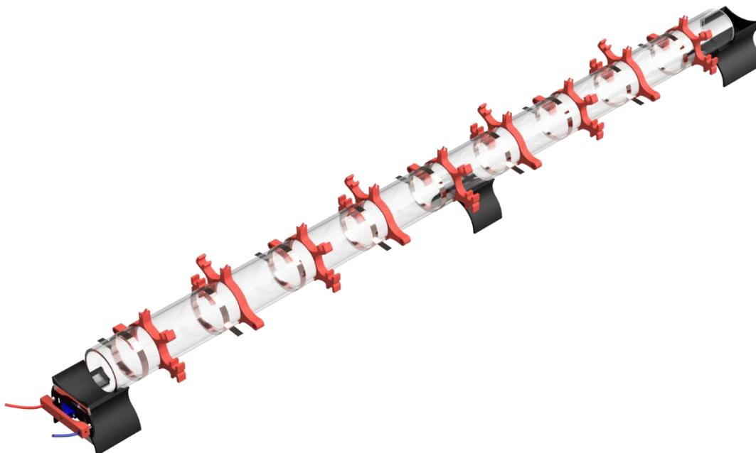
*Clip the HV pylons onto the plexiglass tube with alternating orientation. Leave a bit of space between the HV pylon and the copper loops since the alligator clips have a certain length.*
