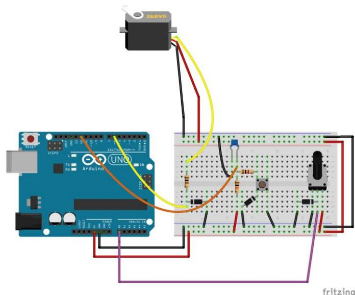
*The control circuit for the linear accelerator is depicted above. A sketch for the Arduino Uno is provided on the S'CoolLAB website. An electronic circuit diagram is provided in the appendix. Omit the LDR-circuit, if you are planning on building the accelerator without light barriers.*
