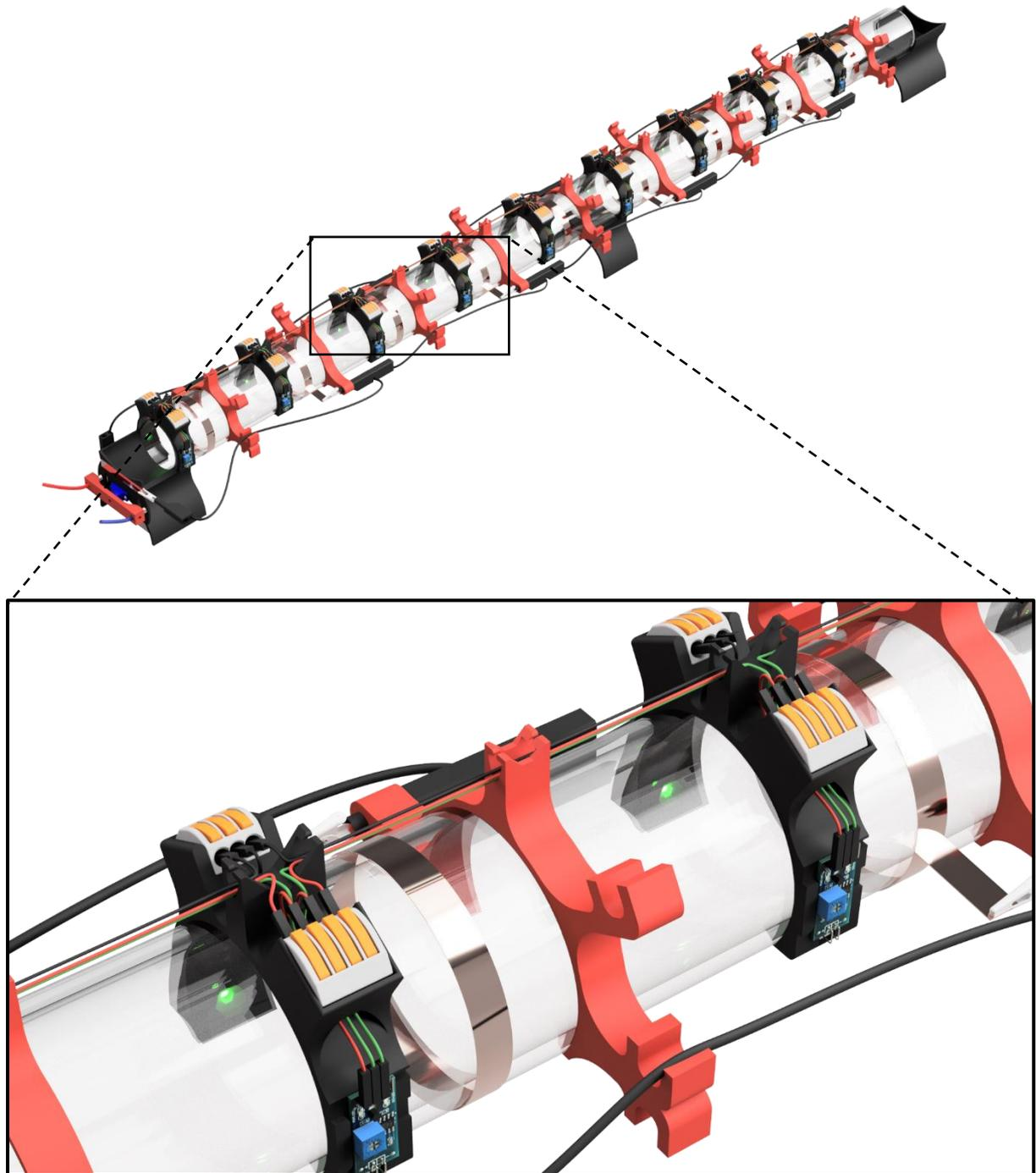
Wire the light barriers according to the schematic. Set the threshold of the Light-dependent resistor modules using the adjustment screw in such a way that the HV switch will be triggered by the Arduino when the photoresistor is shaded from the LED by the ping pong ball.
