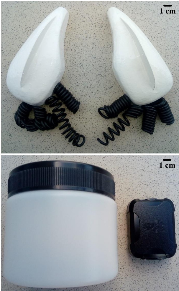
Fig. 2. Prototypes of right- and left-handed P. physalis (top) and components of the satellite-tracked surface drifting buoys used in this study (bottom).
