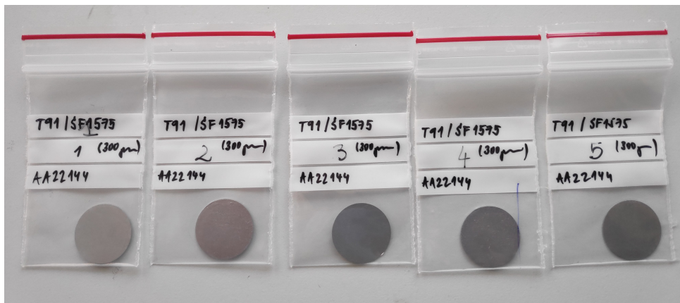
Figure 2.5: T91 steel samples produced by RHP-Technology.
