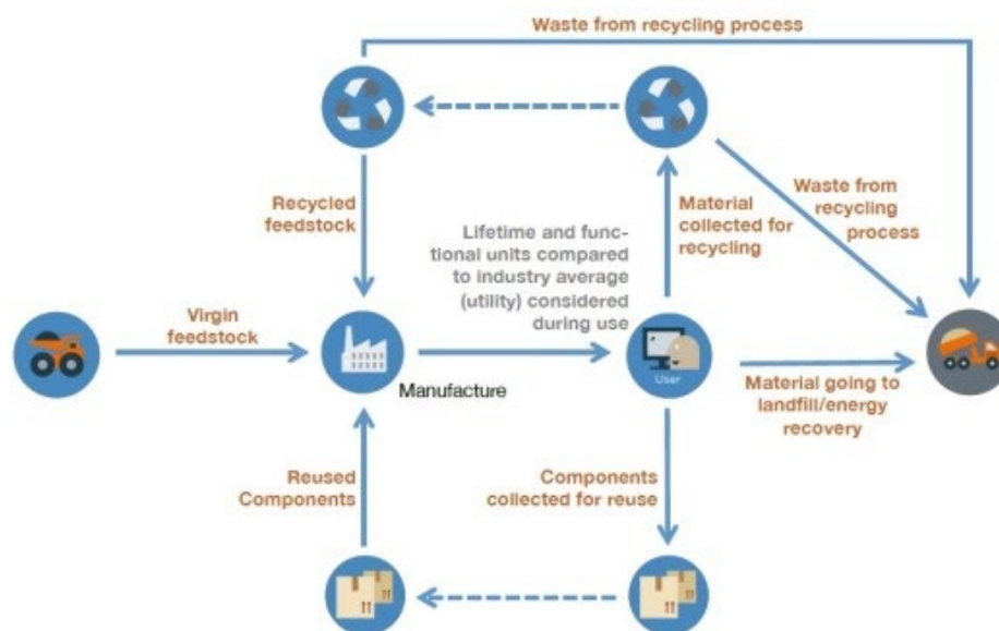
Figure 14.1 The Material Circularity Indicator (Ellen MacArthur Foundation, 2015)
