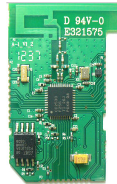
Fig. 2 Front of the processing and radio unit
