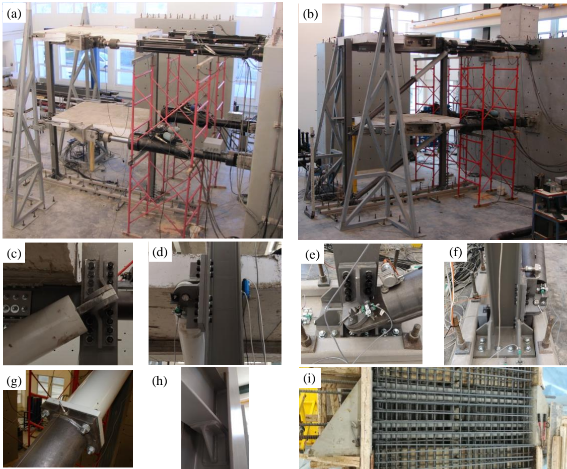
Figure 4. (a) Test setup of the bare test specimen; (b) test setup of the retrofitted test specimen; (c through g) BRB's connection details; (h) beam-to-column connection; (i) slab details.
