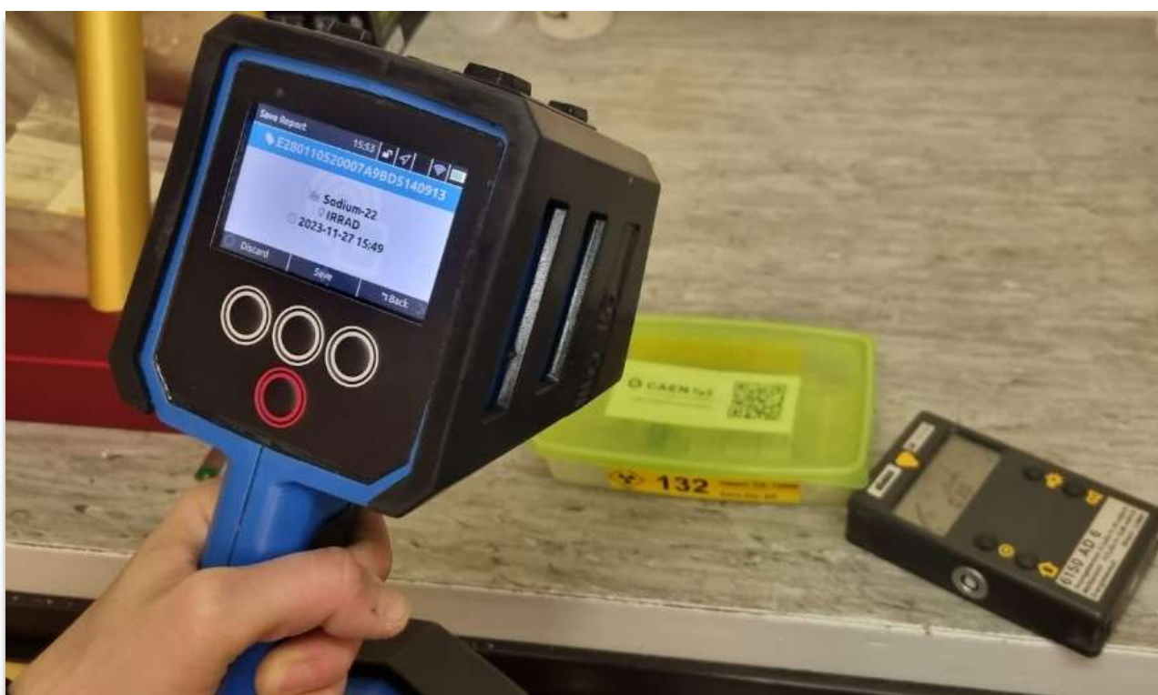
Fig. 6 - CAEN RadHAND device, RFID and radioactive material while performing a measurement.
