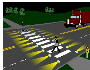
Fig. 8 In-pavement flashing warning lights [9]
