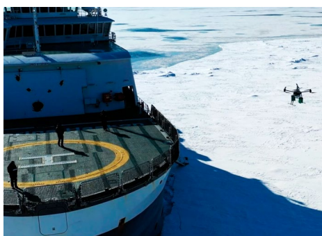
Figure 4-1 Ultra Wideband Snow Sounder (UWiBaSS) on flight during the 2022 CIRFA cruise. Foto: NORCE.
